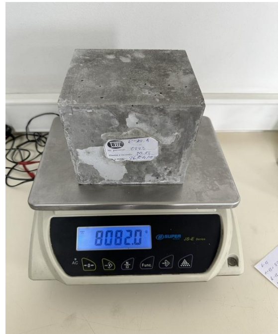
Masa e mostrës R-12.1, M-13 – No Crack
