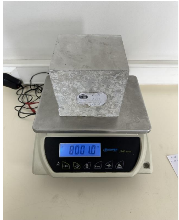
Masa e mostrës R-12, M-13 – No Crack
