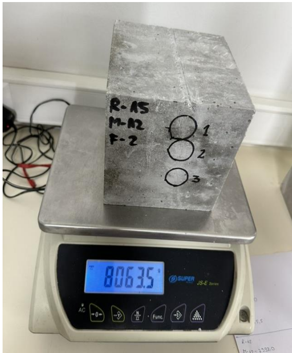
Masa e mostrës R-15, M-12 – Crack
