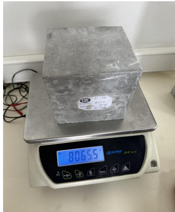
Masa e mostrës R-15, M-13 – No Crack
